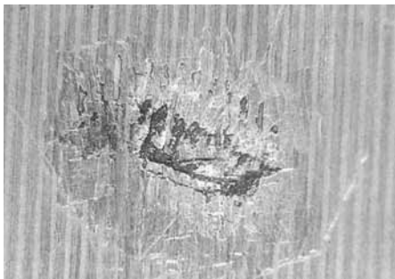
Surface fatigue on ball bearing
